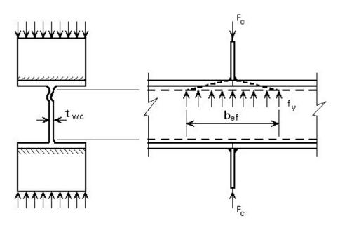
Figure 17 Tests for the determination of b efin the compression zone
