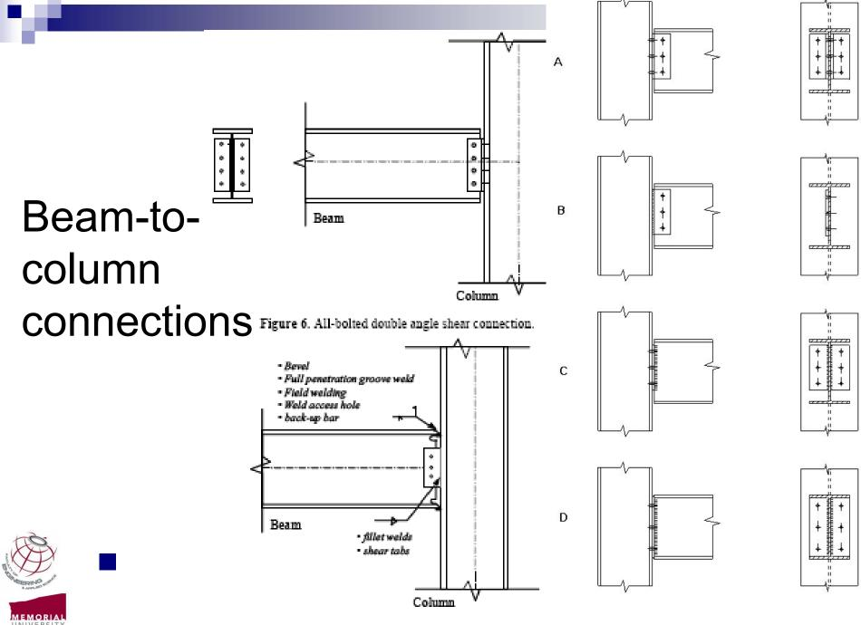
Figure 7. Directly welded flange fully restrained moment com Figure 3 Beam-to-column connections
