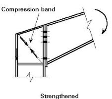
Figure 22 Schematization of the action in the shear zone with tension and compression
