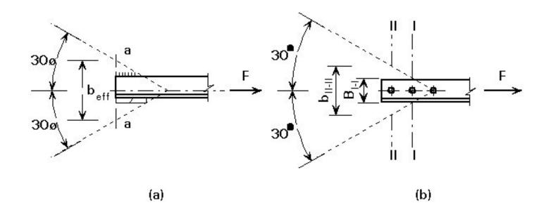
Figure 16 Spread and effective breadth in a welded and a bolted connection
