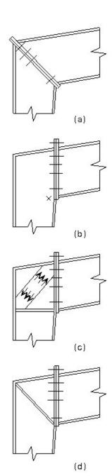
Figure 12 Types of eaves connection
