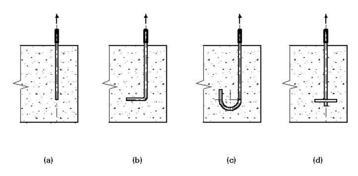
Figure 9 Anchorages of holding down bolts
