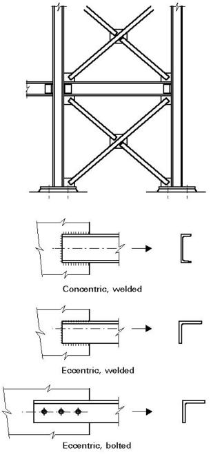
Figure 7 Connection of tension members to gusset plates
