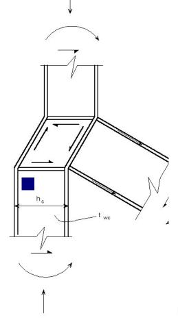
Figure 20 Shear panel of a T-connection
