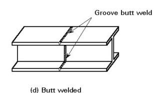
Figure 1 Types of splice arrangements
